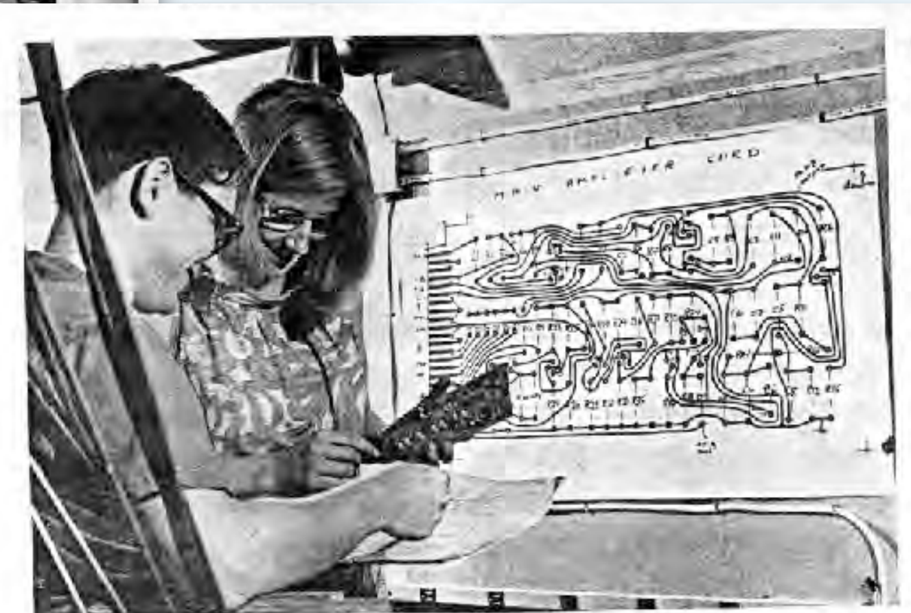
Peter B. Landecker of New York City and Mrs. Cassel, both postdoctoral staff members at Cornell University, examine a main amplifier card that carries the amplification and logic circuits, as diagrammed at the right.
