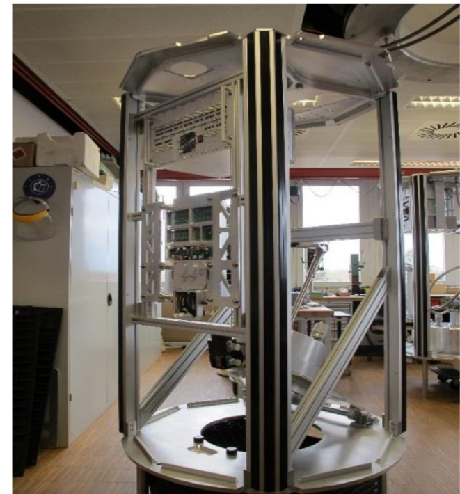
Figure 1: Picture of the UBB Rx in the laboratory. The feed points downwards and is automatically pulled up into the Rx box for storage. In the centre left is the highly integrated EDD front-end unit, which provides control, monitoring, RF conditioning and digitization.
