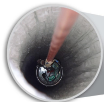
Digital Optical Module (DOM) 5,160 DOMs deployed in the ice
