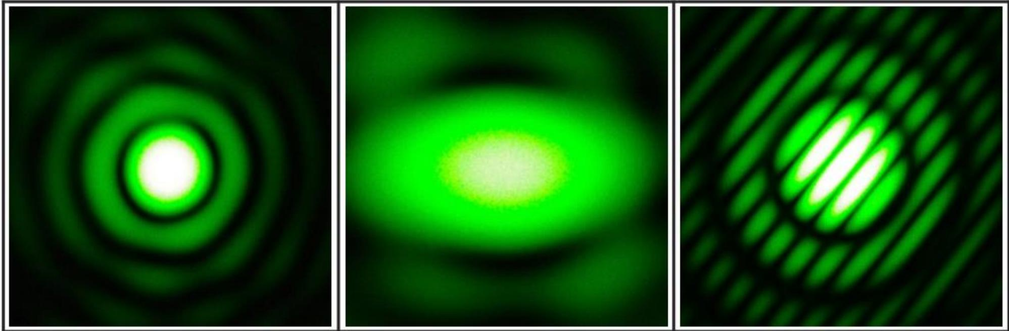
Diffraction patterns with laser light show the [squared] Fourier transforms of some artificial 'stars'. Circular single star; elliptic small single star; binary with equal components. Image widths correspond to ~70 cm in the telescope plane and such baselines are required to retrieve these patterns.
