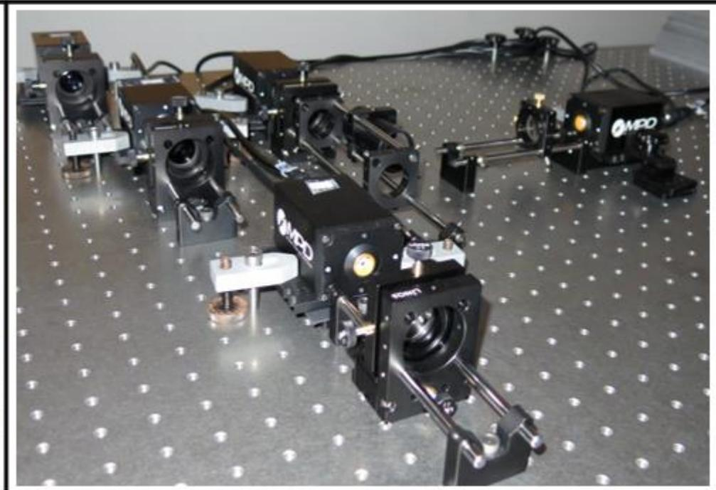
**Left:** Light from a 300 mW  $\lambda$  532 nm laser is randomized through scattering against microscopic particles in a square-top cuvette and focused by a condenser onto artificial 'stars', being apertures in a rotatable holder. **Right:** The 'stars' are observed by an array of small telescopes, each with a photon-counting SPAD detector. 2-D coverage is achieved by rotating the asymmetric source relative to the plane of the telescopes.
