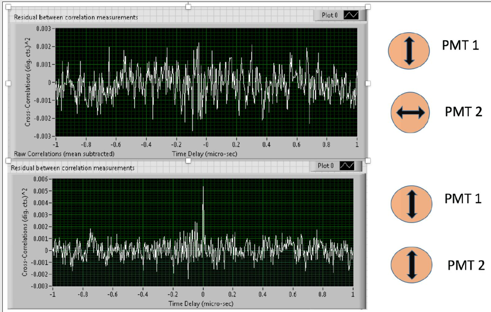
**Temporal coherence from a Hg arc lamp in the laboratory. Upper plot: Non-correlation with perpendicular polarizations. Lower: Observed 2-photon correlation with parallel polarizer configuration.**
