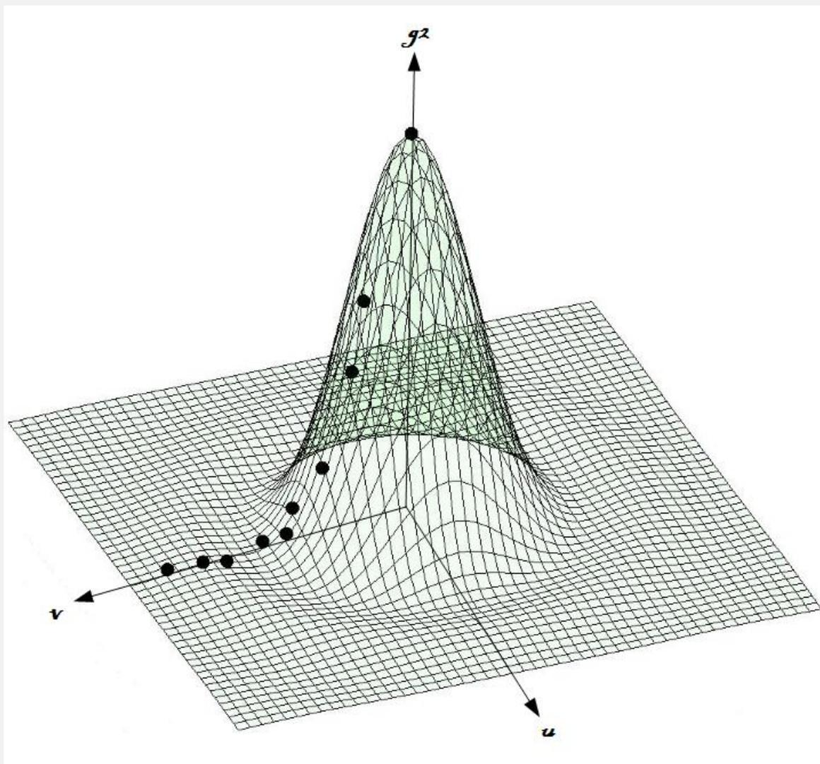
One-dimensional coherence functions sample one particular position angle of the two-dimensional coherence surface, here a sequence of measured points on the surface for an idealized circular aperture.
