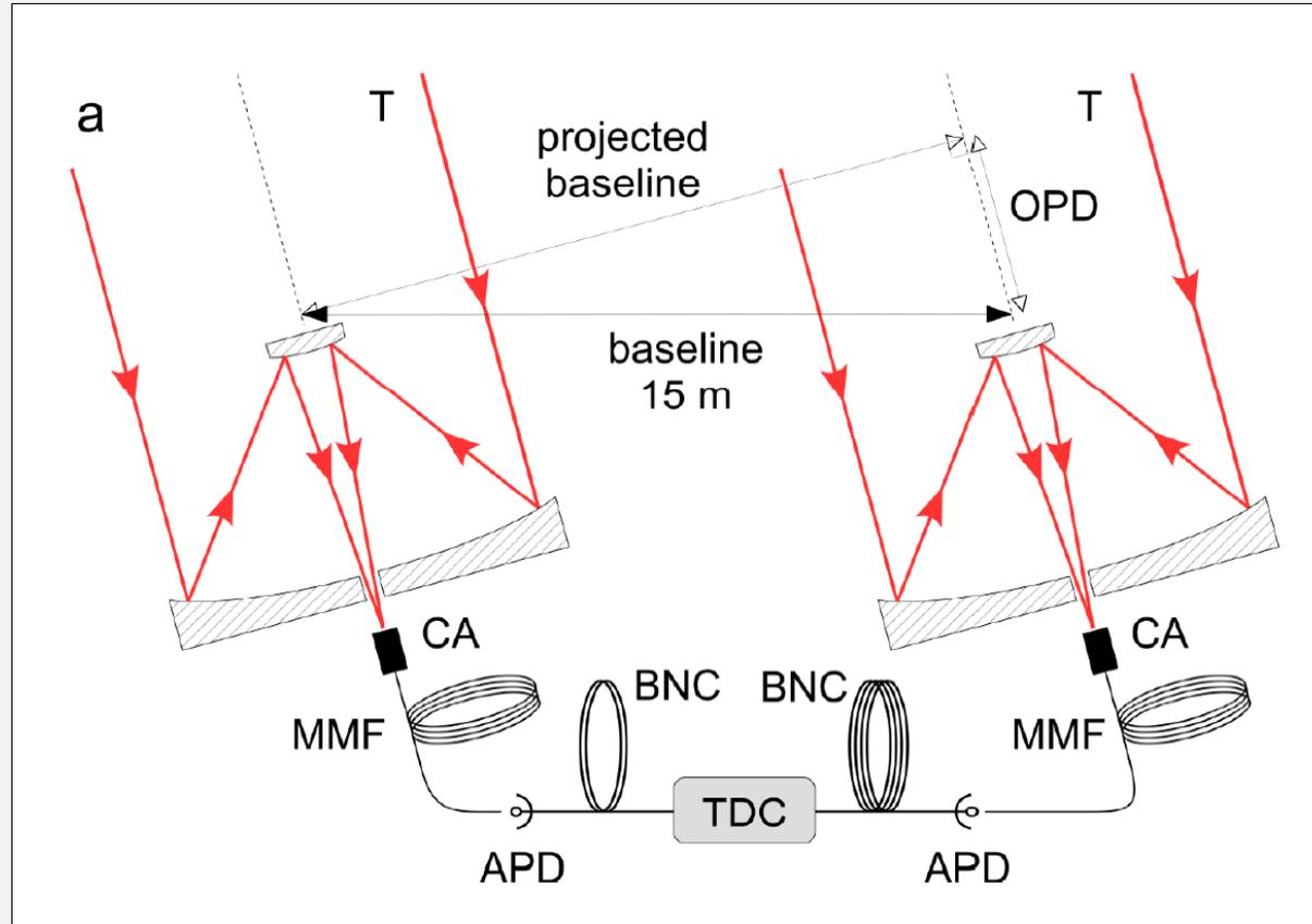
Starlight is collected by two 1-m telescopes and fed into multimode optical fibers (MMF) to an avalanche photodiode (APD), followed by a time-to-digital converter (TDC).
