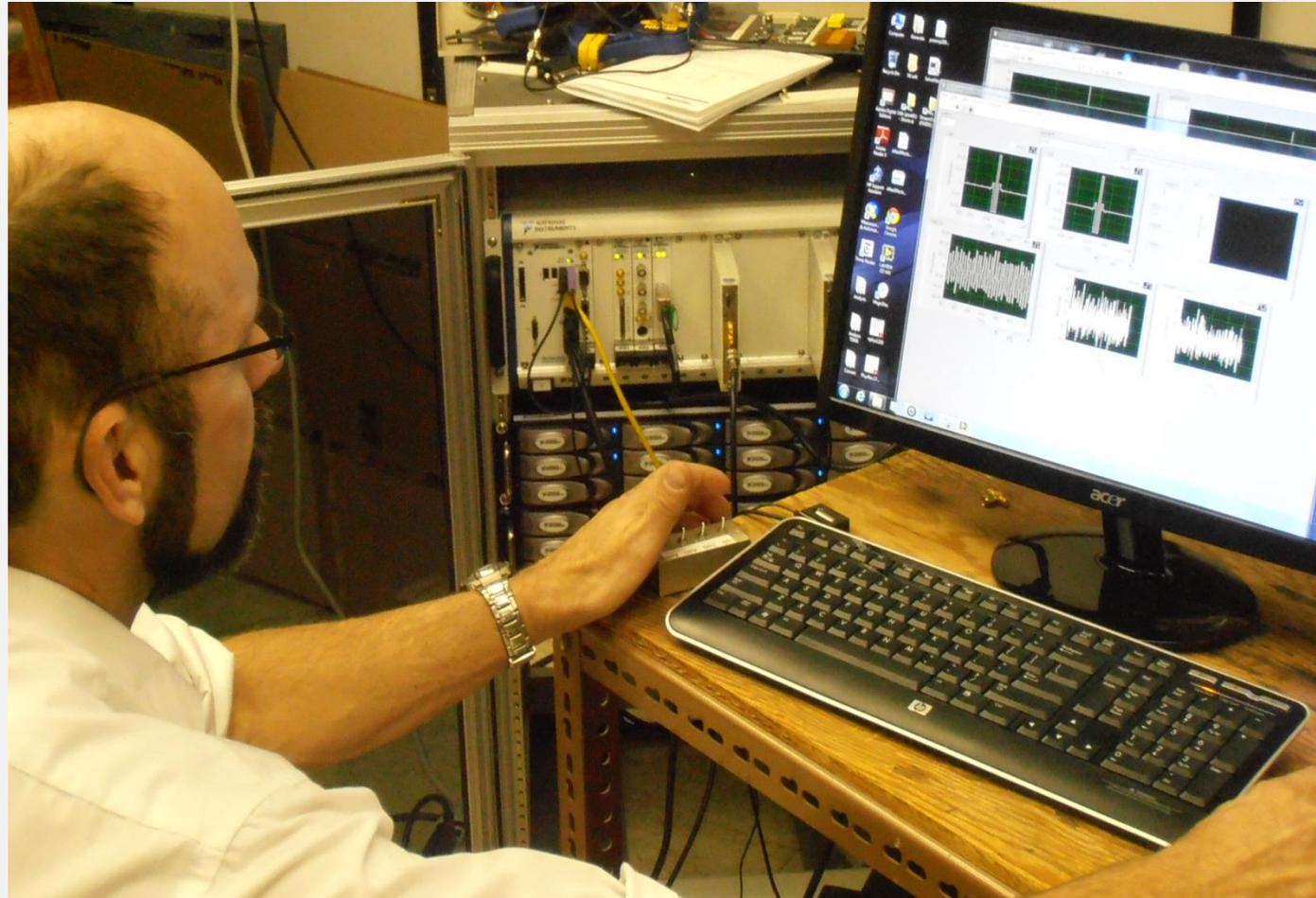
The ongoing VERITAS upgrade includes provisions also for intensity interferometry. Here, David Kieda examines correlation functions computed off-line in electronics for real-time digitization and storage of photomultiplier signals.
