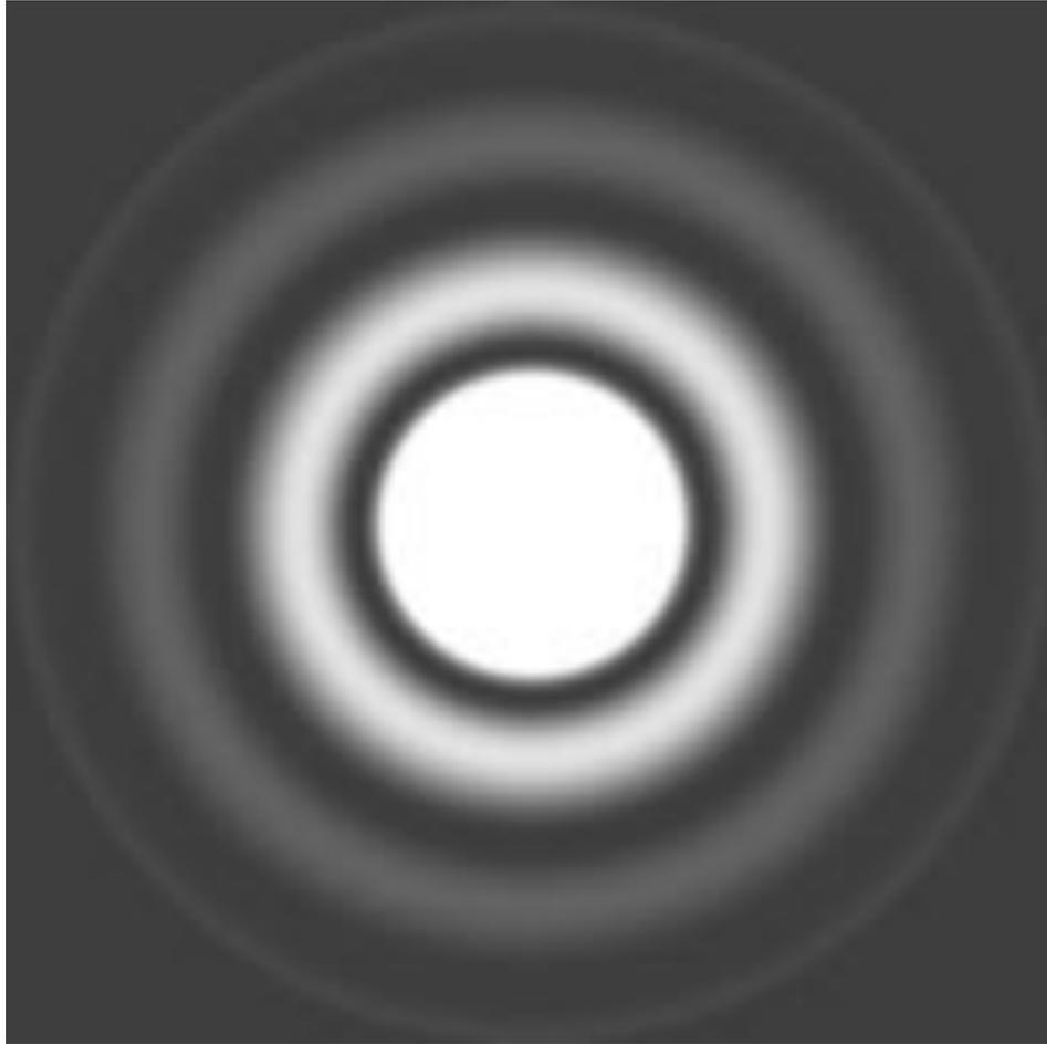
This Airy-disk diffraction pattern is immediately recognized as originating in a circular aperture, although only intensities are recorded.
