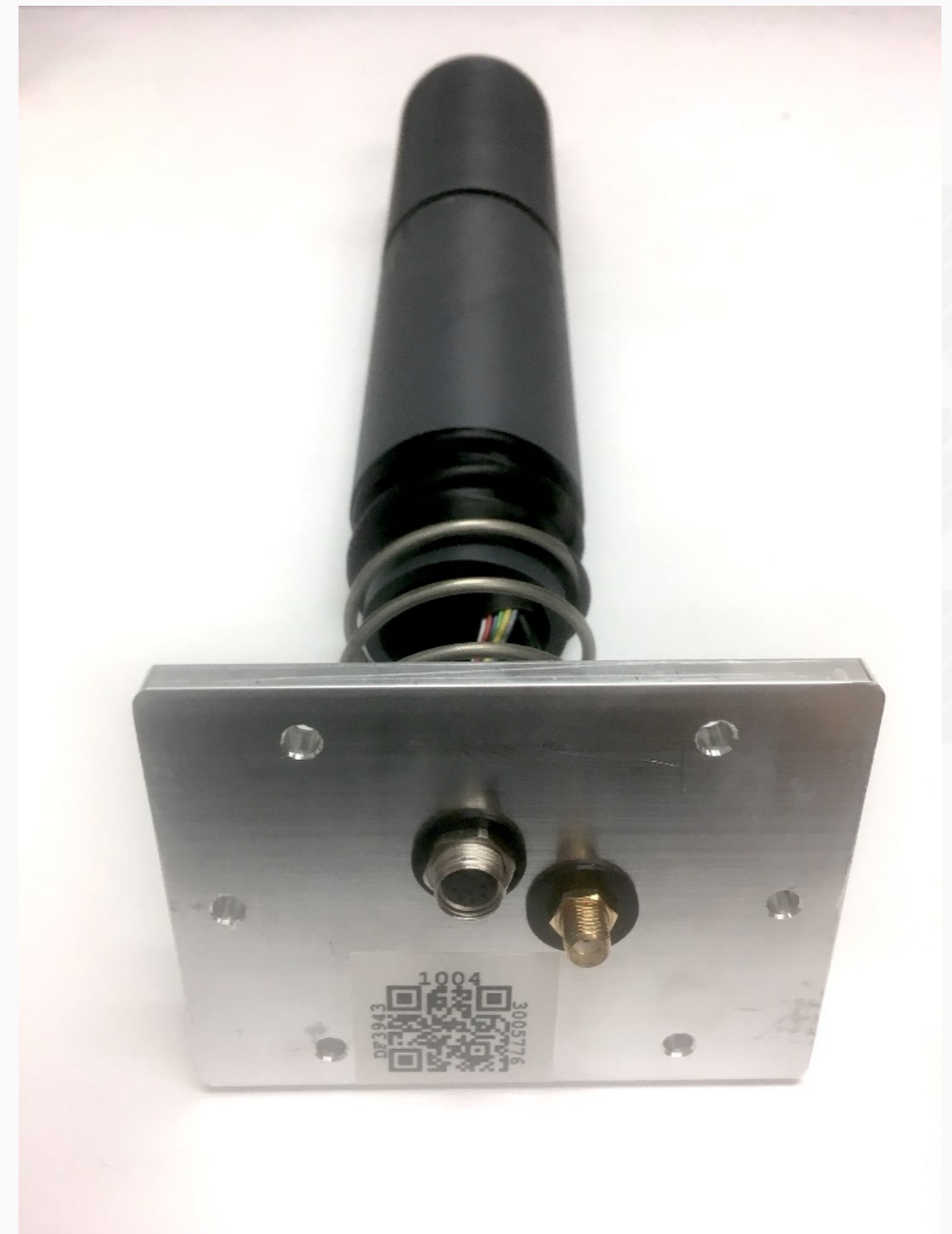
Hamamatsu R9420 PMT fully mounted and soldered
